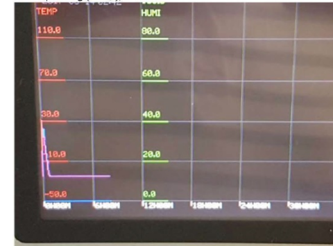
12.2.3 Cooling Test Non-Operating (-25°C), 6 Hours
