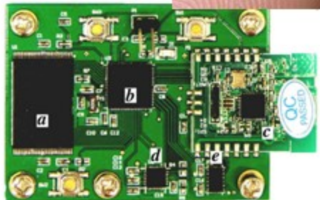
a: Flash Memory b: Microcontroller c: Radio d: MEMS Gyroscope: MPU e: MEMS Accelerometer: A
